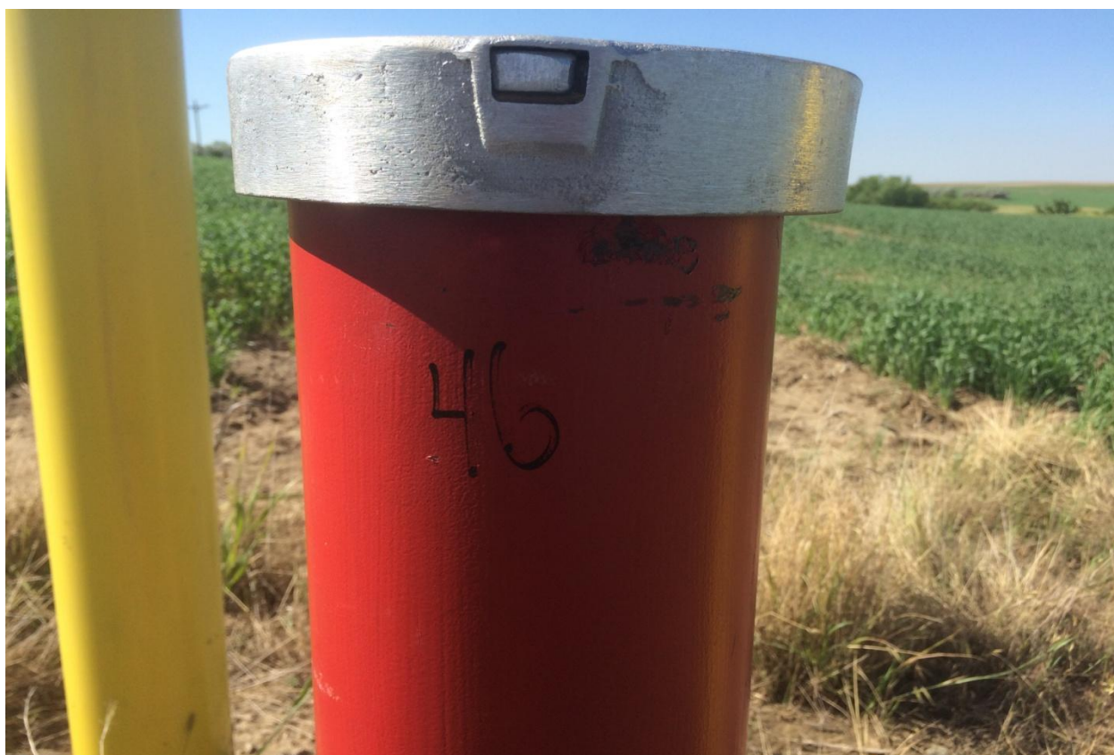
Monitoring well MW-46. Clearly labeled to avoid confusion while collecting samples.
