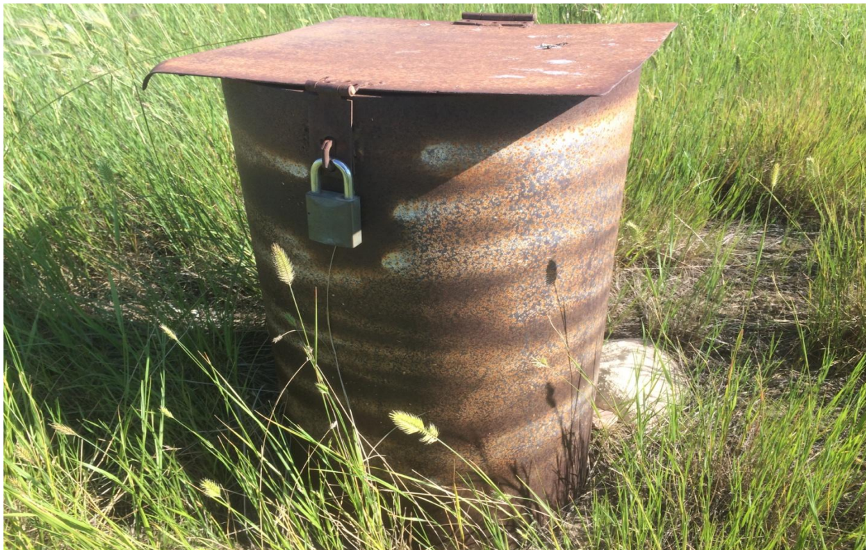
Monitoring well. Properly secured with padlock.
