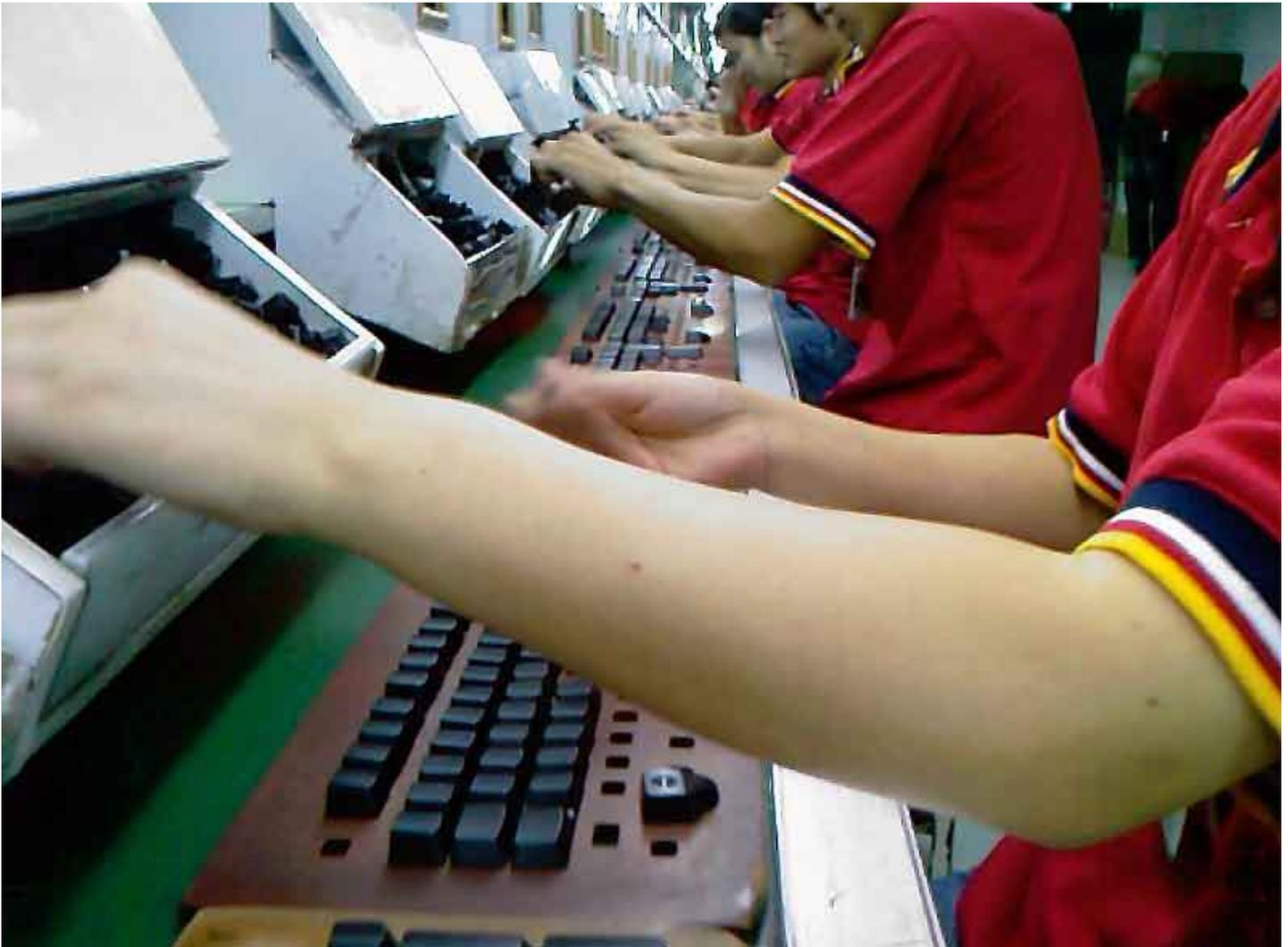
**Keyboard assembly line. Workers sit on hard wooden stools without backrests 12 hours a day racing to complete 500 keyboards an hour. Each worker will complete 35,750 operations a day.**
