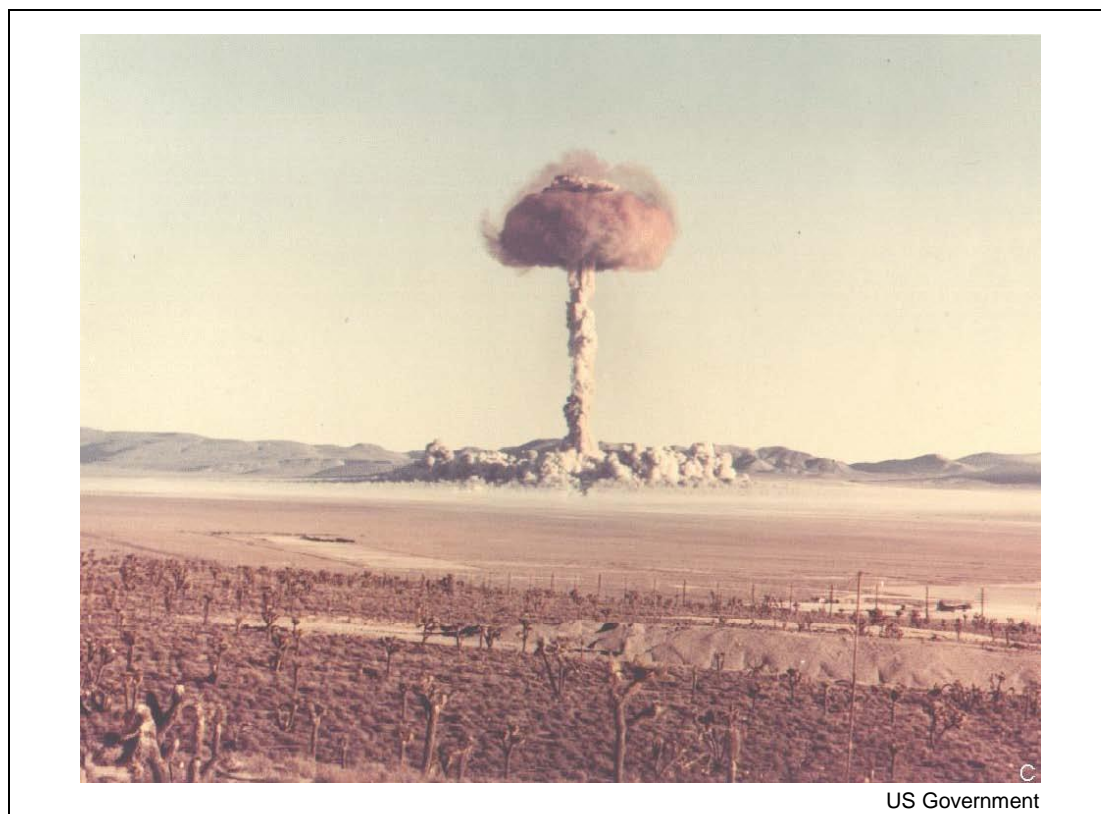
Figure 3-11. The BUSTER CHARLIE detonation was a 14 kt airdrop at the NPG on 30 October 1951. With a height of burst of 1132 ft, the fireball did not touch the ground. The dust stem vacuumed from the desert floor by the rising fireball did, however, reach and penetrate the radioactive mushroom cloud. In this picture, the lighter-toned dust can be seen rising upward through the orange-toned radioactive cloud. The dust is only weakly radioactive at this time. The material in the upper portion of the stem will, however, soon mix with the radioactive debris in the mushroom, and eventually settle back to earth as radioactive fallout.
