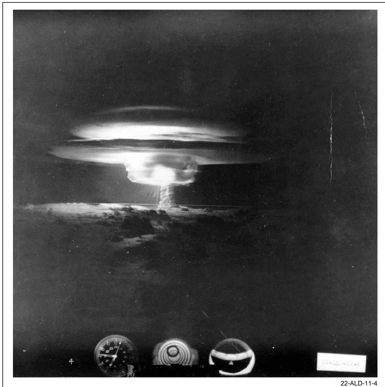
Figure 3-3. BRAVO event, 62 seconds after detonation This image was taken at a distance 50 nm north of GZ from an altitude of 10,000 ft. The lines running upward to the left of the stem and below the fireball are smoke trails from small rockets. At this time the cloud stem was about 4 mi in diameter.
